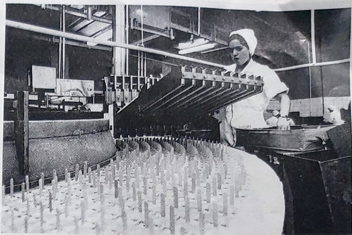
Water ices are an important part of the company's business. Its two Gram Ria machines are kept in full production. Operating this one is Maria Elisete Morgado
